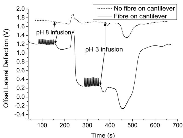
**Fig. 3** Lateral deflection versus time raw data obtained during a single run with and without a PAA fibre attached and stretched by the cantilever. Where the cantilever is attached to a fibre, the fibre is stretched to a strain of 30%. The arrows indicate the starting time of the relevant pH solution infusion.
