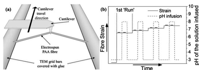
**Fig. 1** (a) diagram of actuation testing apparatus; (b) schematic illustration of the procedure for carrying out constant strain actuation measurements at increasing strains. Each ‘run’ consisted of an initial pre-strain adjustment at pH 3 followed by a small amplitude strain oscillation to determine modulus after which the pH was changed to pH 8 and the small amplitude strain oscillation repeated.
