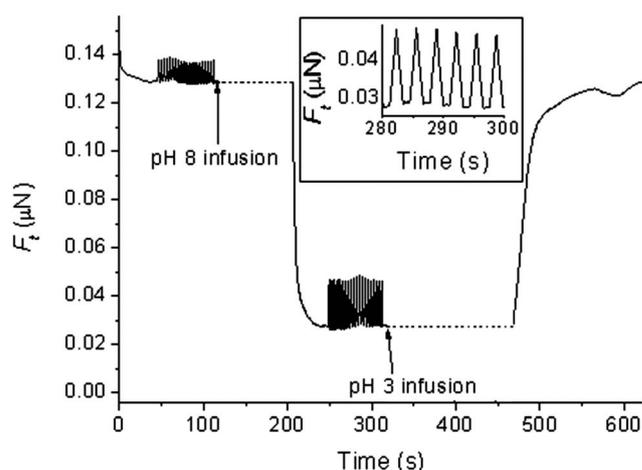
**Fig. 4**  $F_t$  versus time for the same run with a fibre attached that is presented in Fig. 3 and inset showing an expanded portion of the graph that more clearly displays the additional 500 nm cantilever scans. The dashed lines represent where the drift in force due to pH solution mixing was removed from the data.
