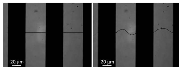
**Fig. 2** Still images from a video taken through an optical microscope of PAA nanofibres UVN<sub>2</sub> treated for 5 min and suspended between the bars of a TEM grid (left) contracted at pH  $\sim$ 3 and (right) swollen at pH  $\sim$ 8. The fibres are traced with a black line for clarity as they are faint in the unaltered picture.
