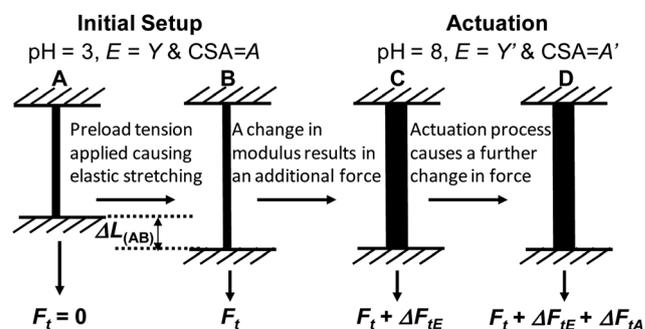
**Fig. 5** Illustration of the PAA fibre held at a constant strain and the components that make up the total force acting on the fibre ( $F_t$ ) upon swelling at pH 8, adapted from.<sup>34</sup> Young's modulus ( $E$ ) and fibre cross-sectional area ( $CSA$ ) are also noted.
