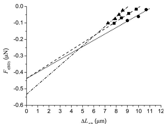
**Fig. 7** Force generated ( $F_{i(BD)}$ ) by the three PAA fibres measured at different initial pre-stretch ( $\Delta L_{AB}$ ).
