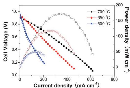
**Fig. 7** Electrochemical performance ( $I$ - $V$  and power density curves) of a prototype cell made of a BZY20 electrolyte film supported on the lab-synthesized anode, measured at 600, 650, and 700 °C.
