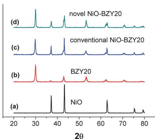
**Fig. 1** XRD patterns of (a) NiO powder, (b) BZY20 powder, (c) NiO-BZY20 composite anode powder prepared by a conventional mechanical mixing process, and (d) NiO-BZY20 composite anode powder prepared by a combustion method.
