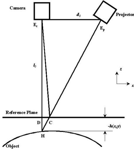
Fig. 1. Optical arrangement of fringe pattern profilometry system
