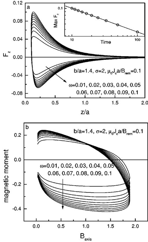
FIG. 8. (a) The vertical magnetic levitation force  $F_z$  (in units  $0.01B_{rem}^2 a^2 / \mu_0$ ) versus the distance  $z$  at  $b/a=1.4$ ,  $\sigma=2$ , and  $\mu_0 J_c a / B_{rem} = 0.1$  for various frequencies at which the PM approaches and recedes from the HTS. The inset shows the relaxation of the levitation force. (b) The corresponding magnetization hysteresis loops.
