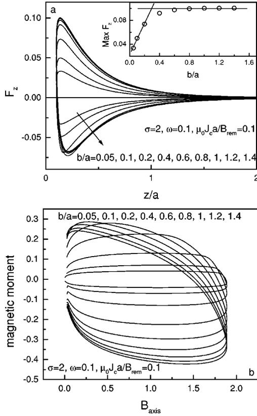
FIG. 5. (a) The vertical magnetic levitation force  $F_z$  (in units  $0.01B_{rem}^2 a^2 / \mu_0$ ) versus the distance  $z$  at  $\sigma=2$ ,  $\omega=0.1$ , and  $\mu_0 J_c a / B_{rem} = 0.1$  for different thicknesses of the superconducting disk. The inset shows the maximum repulsive force as a function of the thickness; the solid lines are a guide for the eyes. (b) The corresponding magnetization hysteresis loops.
