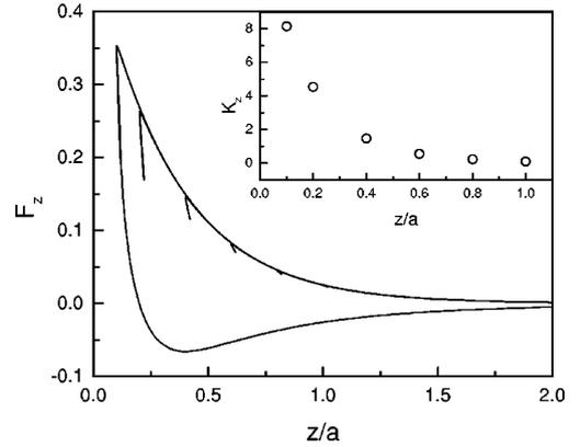
FIG. 9. The vertical magnetic levitation force  $F_z$  (in units  $0.01B_{rem}^2 a^2 / \mu_0$ ) versus the distance  $z$  at  $b/a=1.4$ ,  $\sigma=100$ ,  $\omega=0.1$  and  $\mu_0 J_c a / B_{rem} = 0.1$ . Minor force loops at different distances  $z$  are shown with a amplitude  $\delta z = 0.02a$ . The inset shows the stiffness of the system.
