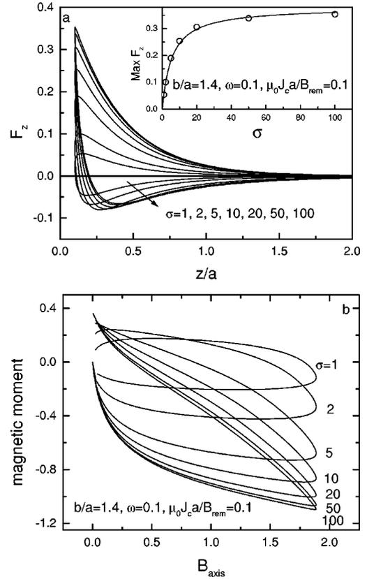
FIG. 6. (a) The vertical magnetic levitation force  $F_z$  (in units  $0.01B_{rem}^2 a^2 / \mu_0$ ) versus the distance  $z$  at  $b/a=1.4$ ,  $\omega=0.1$  and  $\mu_0 J_c a / B_{rem} = 0.1$  for various creep parameters of the superconducting disk. The inset shows the maximum repulsive force as a function of  $\sigma$ ; the solid line is a guide for the eyes. (b) The corresponding magnetization hysteresis loops.
