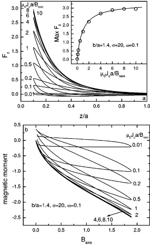
FIG. 7. (a) The vertical magnetic levitation force  $F_z$  (in units  $0.01B_{rem}^2 a^2 / \mu_0$ ) versus the distance  $z$  at  $b/a=1.4$ ,  $\sigma=20$  and  $\omega=0.1$  for different critical current densities of the superconducting disk. The inset shows the the maximum repulsive force as a function of  $J_c$ ; the solid line shows the fit  $F_z = 3.31(\mu_0 J_c a / B_{rem}) / [0.93 + (\mu_0 J_c a / B_{rem})]$ . (b) The corresponding magnetization hysteresis loops.
