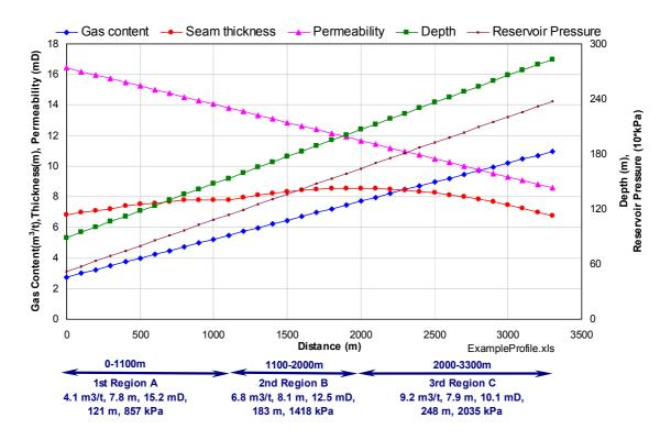
Fig. 4 Example Gas Reservoir Parameter Profile Along an Intended Gate Road
