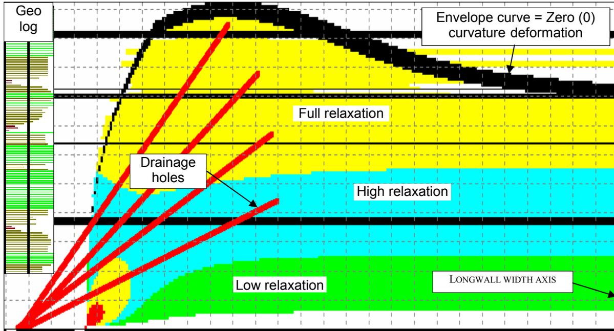
Fig. 4 Roofgas<sup>®</sup> version 3.0 output using rock strata curvature enforcement model - vertical cross section of half of the longwall with strata relaxation & gas release zones for 250 m distance behind the face
