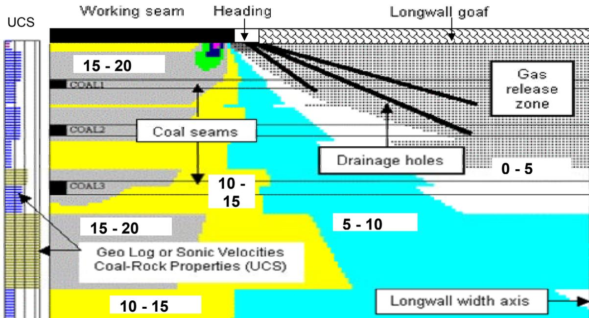
Fig. 5 'Floorgas'<sup>®</sup> output - vertical cross section of half of the longwall with single entry heading, strata relaxation and gas release shape and vertical stresses (MPa) as well as projected down holes
