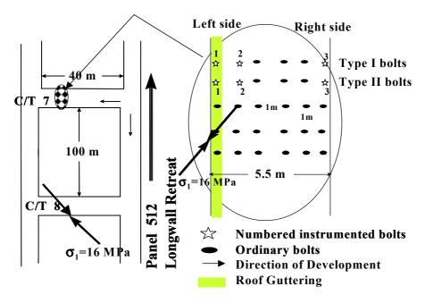
Fig. 8 Plan of instrumented site
