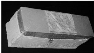
Fig. 1. Flattened bolt surface
