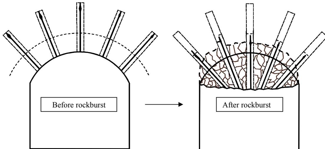
**Fig. 4 Depiction of how the Cone bolt contains broken ground after a rockburst. (not to scale)**
