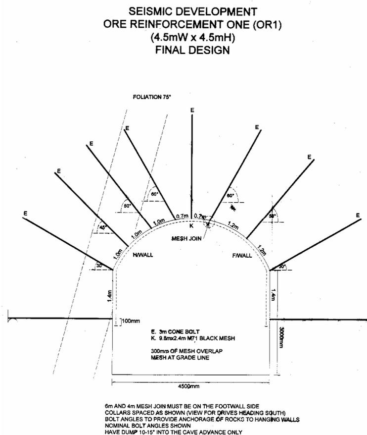
**Fig. 3 Cone bolting pattern for ore drives**
