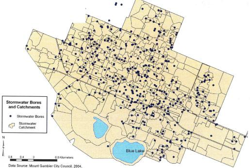
Figure 1 Stormwater draining wells and catchments areas in the City of Mount Gambier (Wolf et al., 2006)
