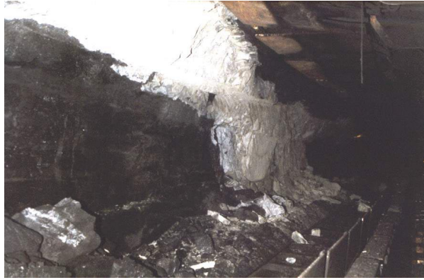
Plate 2. An igneous dyke (white) on some 2-3m thick running near parallel to a longwall face line, AFC at base and chocks to right.
