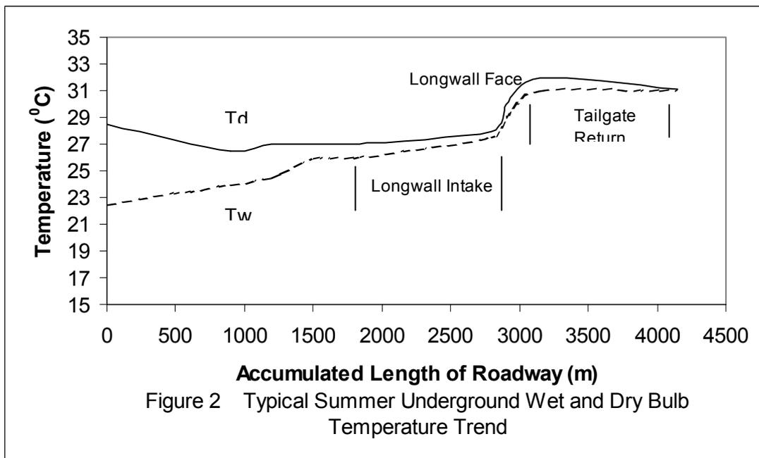
With increasing lengths of longwall panels the intake air is approaching 26°C to 27°C wet bulb at the longwall stage loader. There is very little margin available before heat management action must be implemented on the longwall face.
