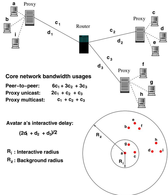
Fig. 2. Network bandwidth usages and interactive delay calculation
