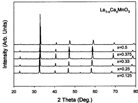
FIG. 1. X-ray diffraction patterns of  $\text{La}_{1-x}\text{Ca}_x\text{MnO}_{3+\delta}$  oxides.
