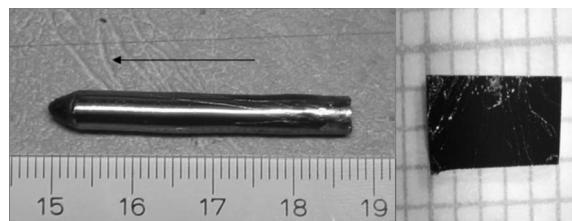
FIG. 1. (Left) As-grown single crystal of \alpha - \text{NaCoO}_2 and (right) the cleaved crystal from the last grown part of the ingot.
