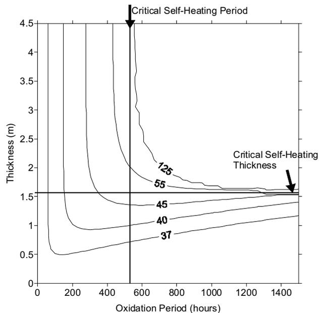
FIG 6 - The impact of pile thickness variations (peak pile temperature °C) on development of a heating.
