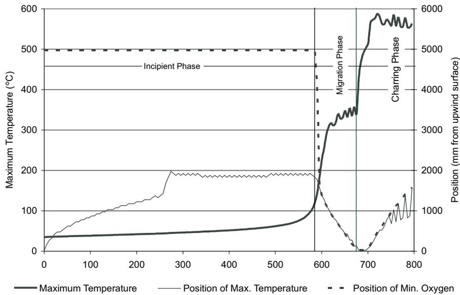
FIG 5 - Base case heating development – temperature and oxygen.
