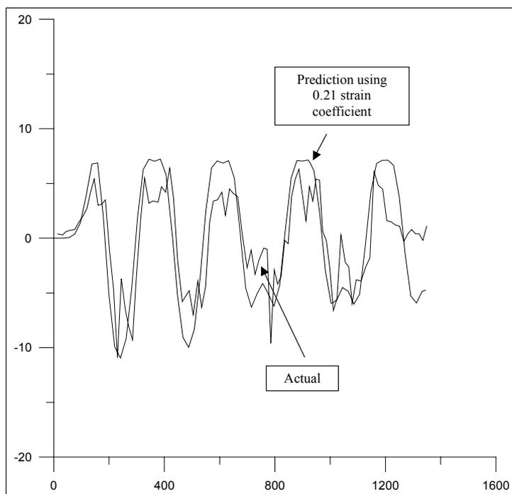
**FIG.11 - Calibration of strain at Mine B**
