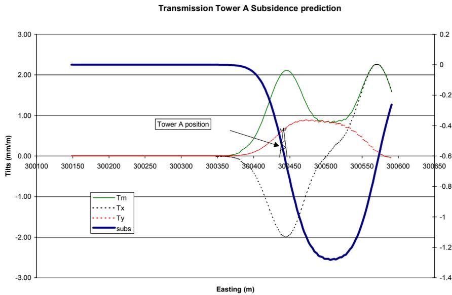
FIG. 4 - Tilt and subsidence at the location of a transmission tower, with changing longwall position
