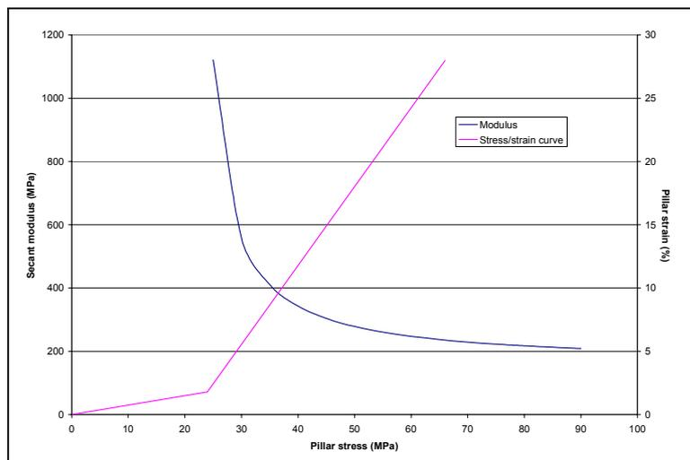
**FIG. 7- Deformation data of Southern Coalfields coal pillars**
