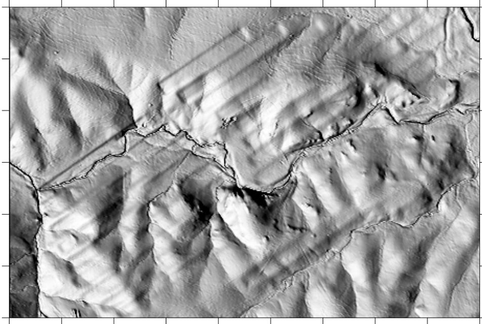
**FIG. 14- Shaded relief surface of subsided topography**
