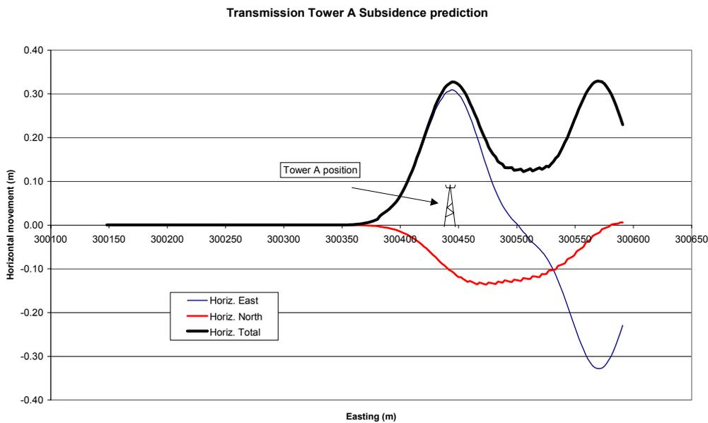
FIG. 5 - Horizontal movement above retreating longwall
