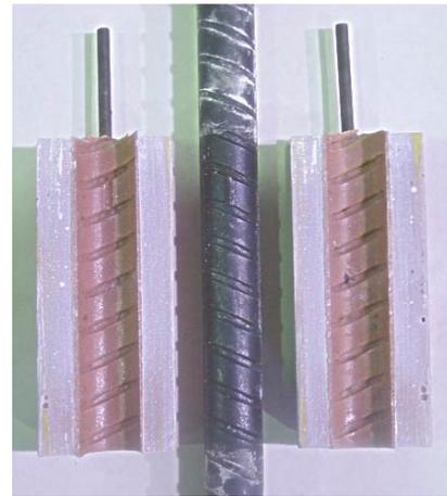
FIG. 9 - Resin bolt separation after Post encapsulation
