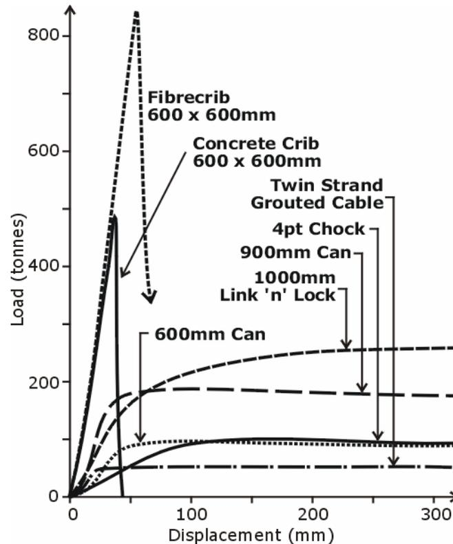
FIG. 6 - Comparative load/displacement of various standing supports
