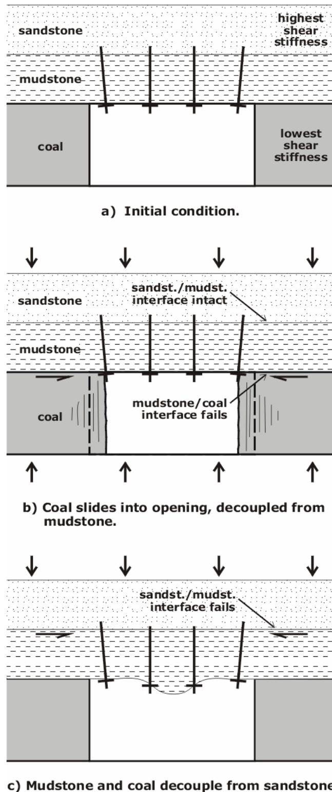
**FIG. 4 - Variation in style of roadway behaviour as a consequence of slip along differing interfaces**
