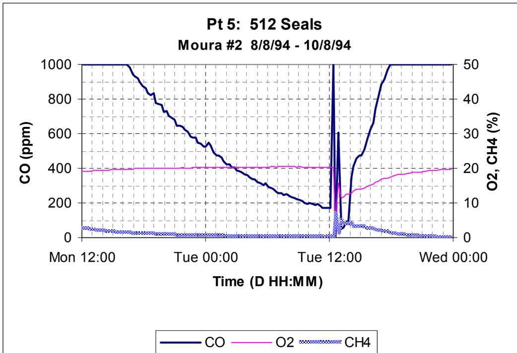
FIG. 1 - Graphs of gas monitoring at Moura No 2
