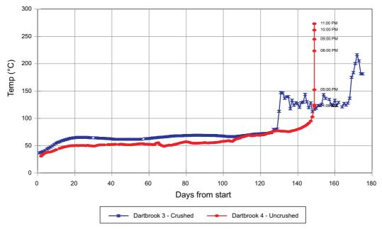
FIG 3 - Temperature time plots for large-scale oxidation tests (Cliff et al, 2000).
