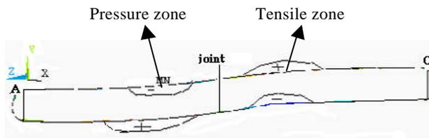
Fig 8 - Tensile and pressure stresses zones around the bolt
