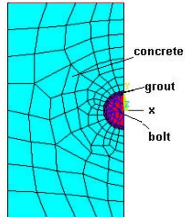
Fig 3 - Three-dimensional image of the numerical model
