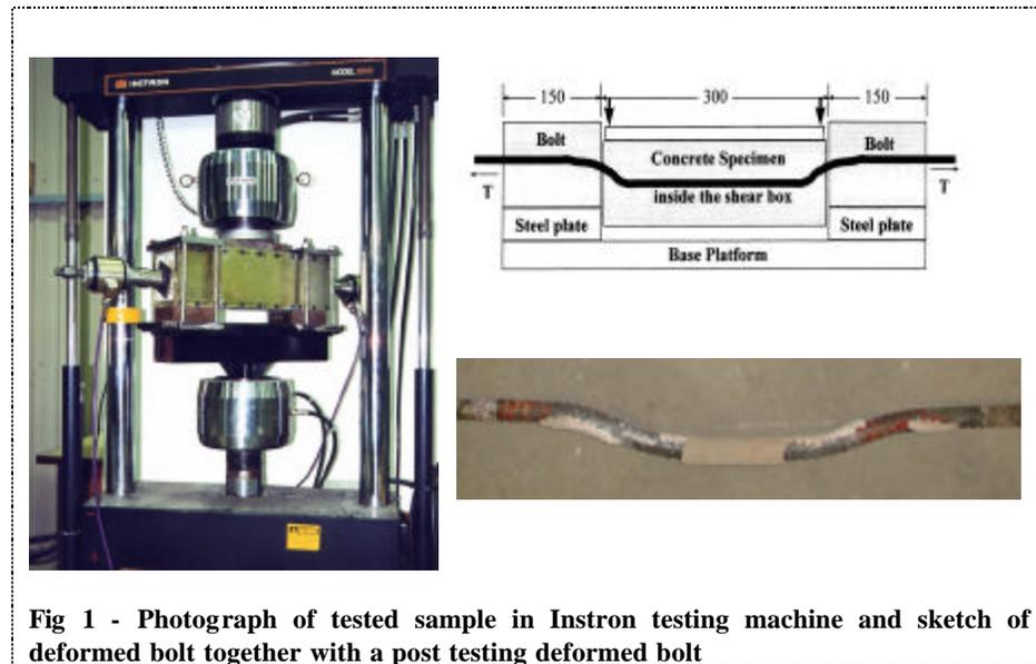
Tests were made with axial confining loads of 20, 50 and 80 kN respectively. The development of shearing loads was examined with respect to the surface profile configuration of the bolt used. Shearing tests were conducted in two different concrete blocks of 20 MPa and 40 MPa strength. Figure 2 shows a typical Shear load and displacement profiles of three different bolts cast in 40 MPa concrete.
