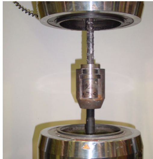
Fig 7 – Pull tests arrangement
