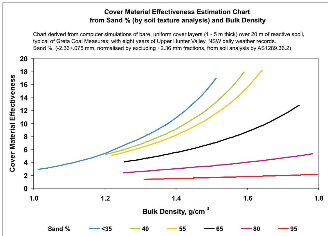
FIG 2 - Plot of the relative effectiveness of cover materials as function of their soil analysis and the degree of compaction.
