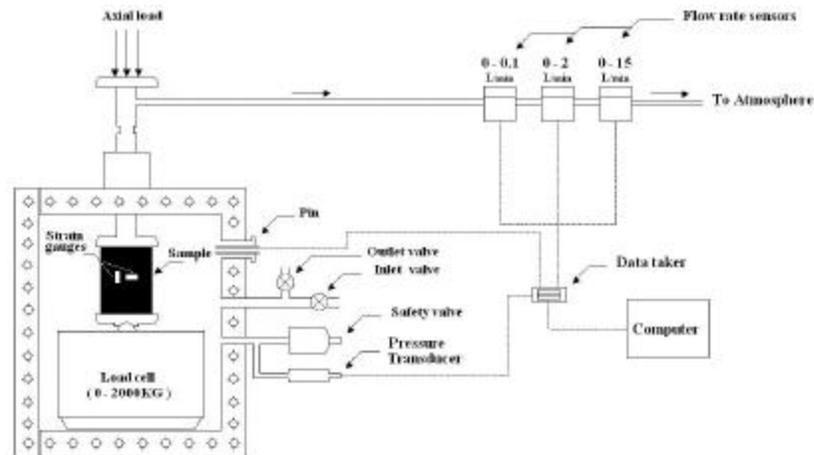
**Fig 1 - Schematic layout of the permeability test equipment**
