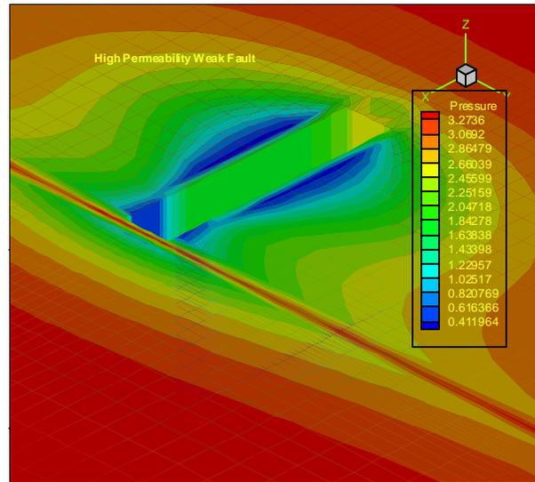
Fig 8 - Pressure distribution in weak fault behind face
