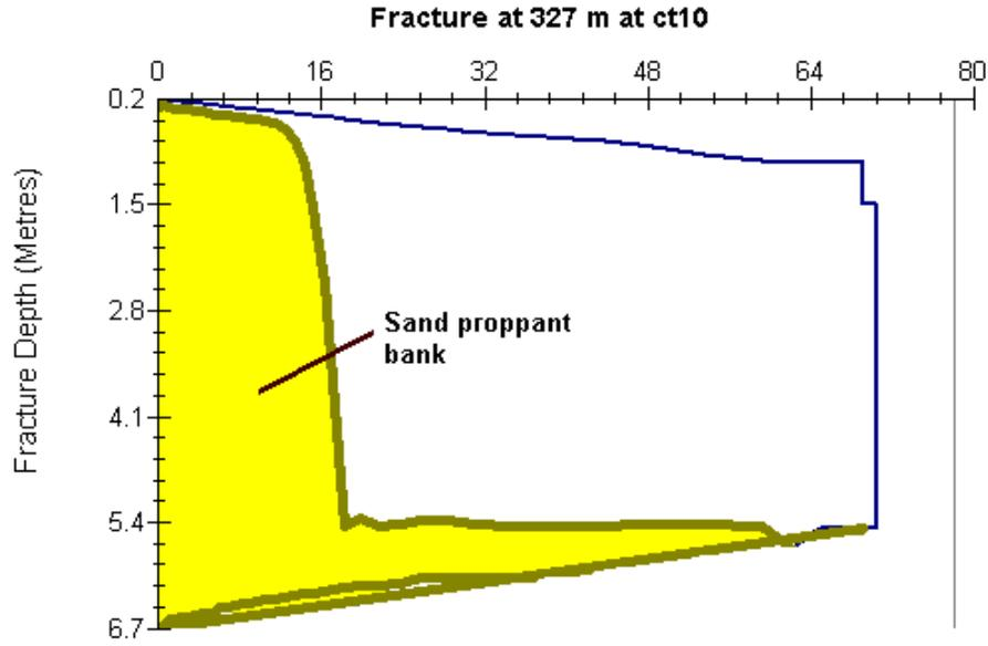
**Fig 5 - The model-predicted proppant bank for the treatment at 327 m at cut-through 10. 160 kg of sand was placed in this treatment.**
