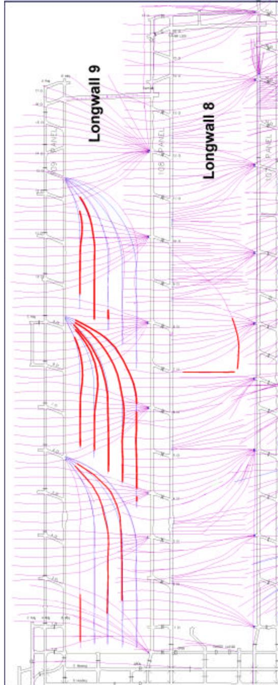
**Fig 1 - Longwall 9 with hydraulic fractured holes indicated.**
