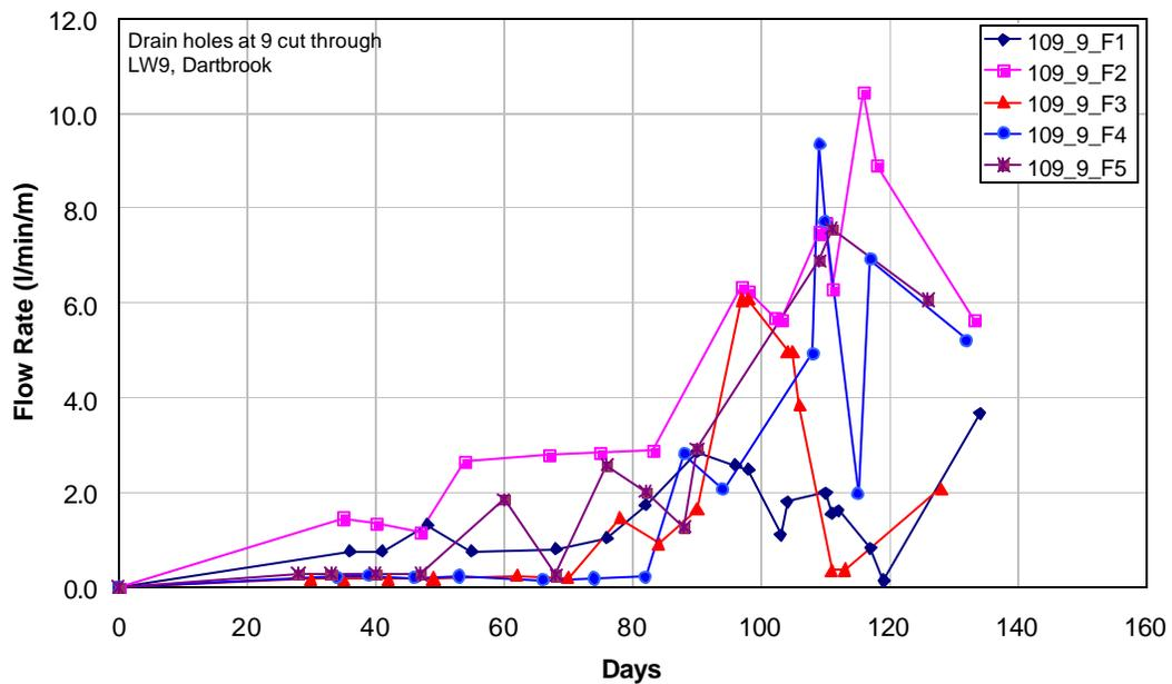
Fig 8 - Specific gas rate from drain holes drilled at cut-through 9. All holes were stimulated.
