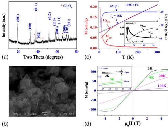
FIG. 1. (Color online) The XRD pattern and index (a) SEM image (b) and magnetic behaviors of cobalt hydroxide nanosheets, M-T,  $1/\chi$ -T, and  $\delta M/\delta T$ -T curves under 100 Oe FC; the insert show the M-T and  $1/\chi$ -T curves under ZFC (c), selected M-H loops at temperatures of 3, 10, 20, and 100 K (d).
