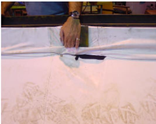
**Fig 3 - Fabric A failure at plate zones**
