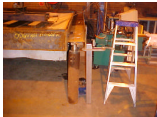
Fig 10 - Buckling of the test frame under load
