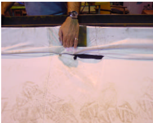
Fig 3 - Fabric A failure at plate zones
