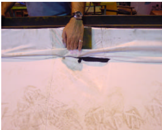
Fig 3 - Fabric A failure at plate zones
