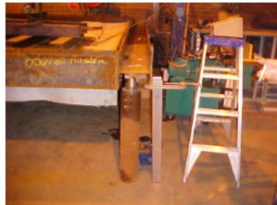
Fig 10 - Buckling of the test frame under load
