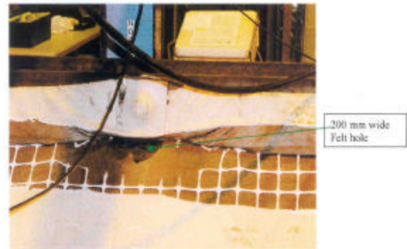
Fig 5 – 280mm lateral width of the torn felt around the central plate @ 68 kN load (total applied load – 0.795t)
