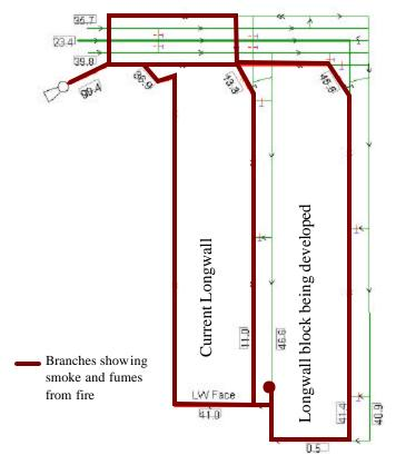
Fig 9 - Smoke progression with diagonal connection
