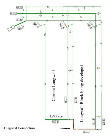
Fig 7 - A typical diagonal connection in Australian coal mine
