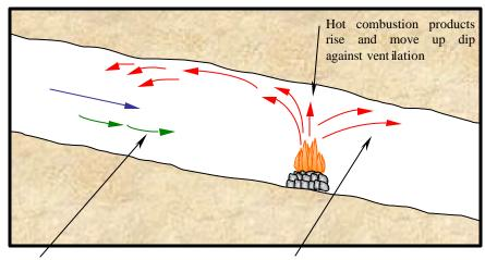
Upwind, the combustion products cool or are mixed into general body of air to travel back to the fire Hot combustion products stay against roof and move down dip at slower speed than the general body
