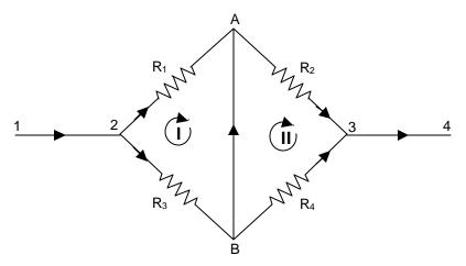
Fig 6 - Ventilation network circuit - Wheatstone bridge
