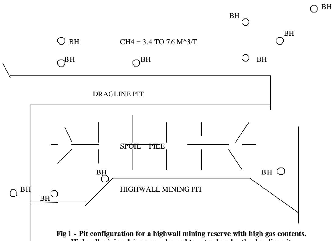
**Fig 1 - Pit configuration for a highwall mining reserve with high gas contents.
