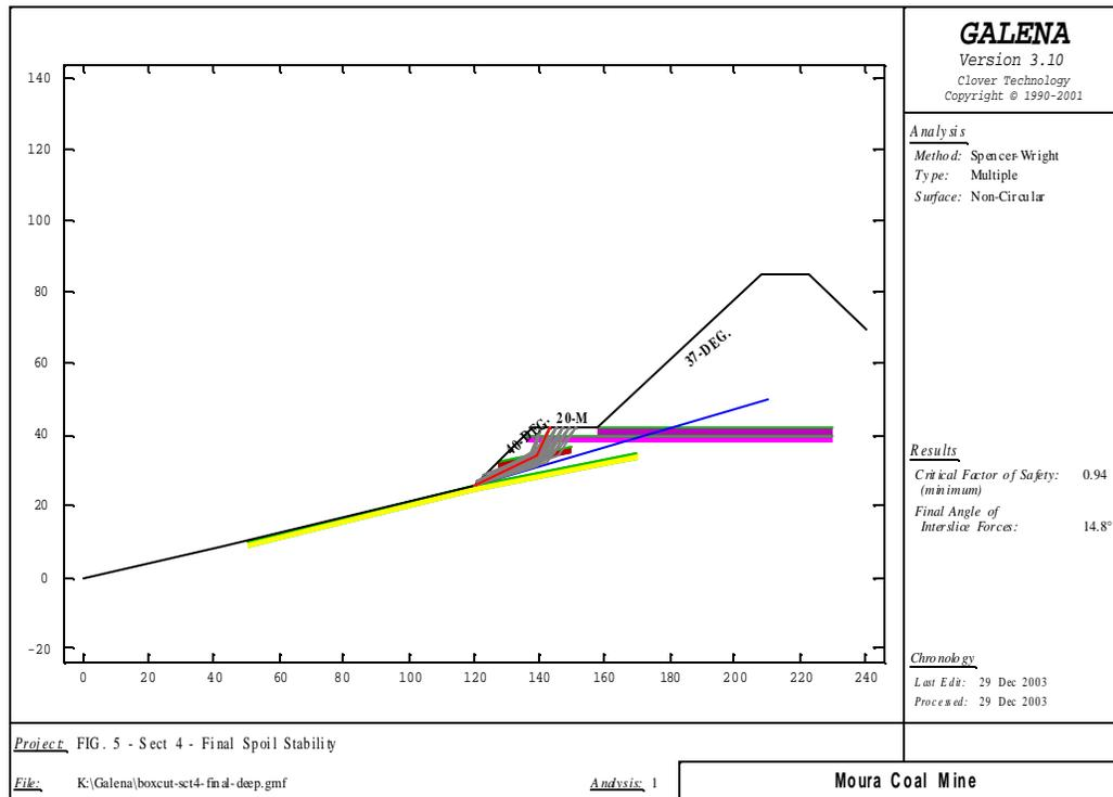
**Fig 3 - Example of slope stability analysis indicating sh allow failure in low wall.
