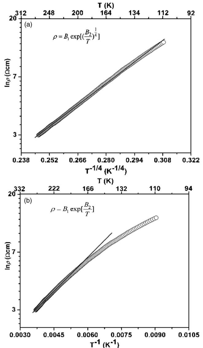
FIG. 3. Fittings of logarithm of electrical resistivity ( $\rho$ ) vs temperature ( $T$ ) for sample  $\text{In}_{1.95}\text{Ni}_{0.05}\text{O}_3$  applying (a) variable range hopping and (b) nearest neighbor hopping conduction models.
