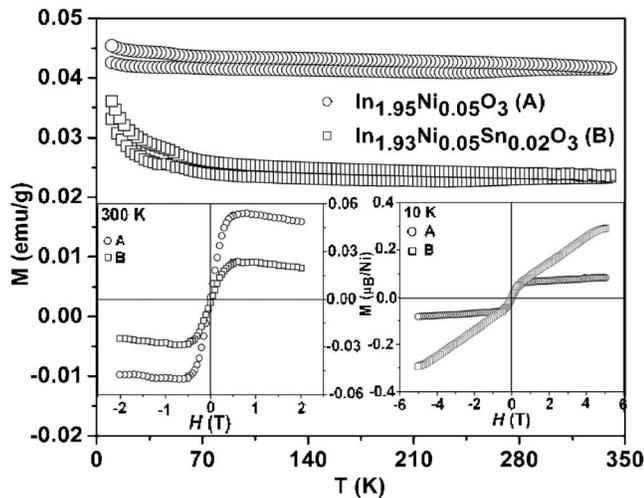
FIG. 4. Magnetization ( $M$ ) as a function of temperature ( $T$ ) for samples Ni-doped  $\text{In}_2\text{O}_3$  (open circle) and Ni-doped ITO (open square) under 2000 Oe applied magnetic field. Insets:  $M$ - $H$  loops of the same samples at 300 K (left) and 10 K (right).
