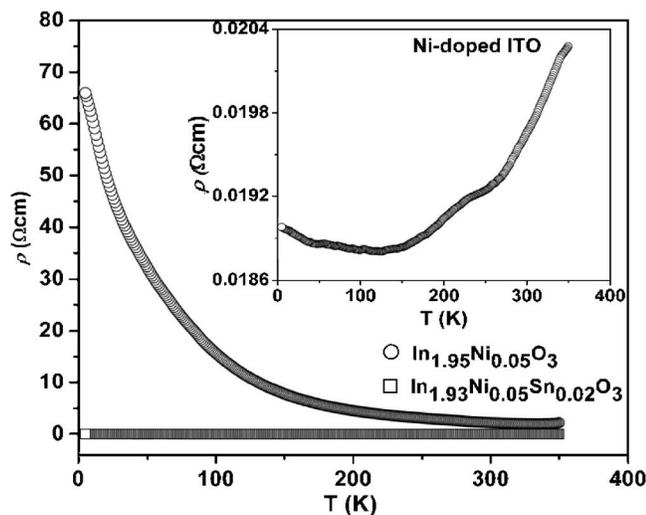
FIG. 2. Electrical resistivity ( $\rho$ ) vs temperature ( $T$ ) for  $\text{In}_{1.95}\text{Ni}_{0.05}\text{O}_3$  (open circle) and  $\text{In}_{1.93}\text{Ni}_{0.05}\text{Sn}_{0.02}\text{O}_3$  (open square). The inset represents magnified view of  $\rho$ - $T$  curve for Ni-doped ITO sample.
