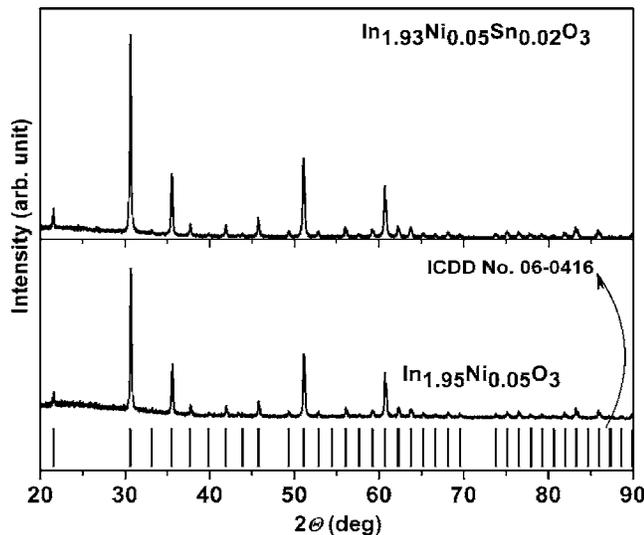
FIG. 1. X-ray powder diffraction patterns of pulverized  $\text{In}_{1.95}\text{Ni}_{0.05}\text{O}_3$  and  $\text{In}_{1.93}\text{Ni}_{0.05}\text{Sn}_{0.02}\text{O}_3$  pellets. The inset shows reference peaks for  $\text{In}_2\text{O}_3$  phase from ICDD Card No. 06-0416.
