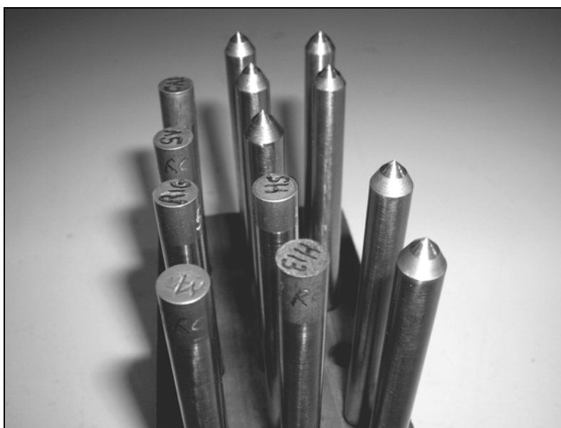
Figure 2 - Sample of some of the steel styli used in the study
