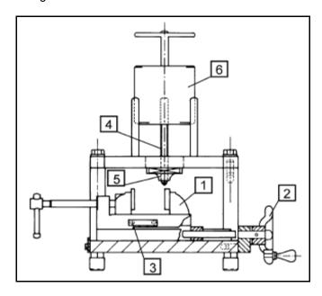
Figure 1 - Cerchar apparatus (after West, 1989)
