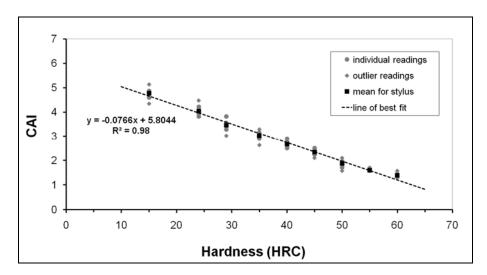
Figure 6 - Effect of steel hardness on CAI with a constant steel type
