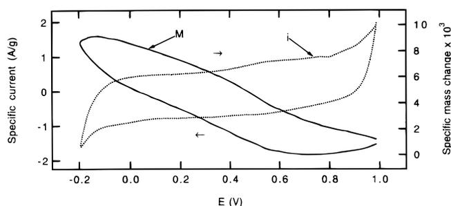
**Figure 5.** Specific current (current/sample mass) and specific mass (mass change/sample mass) as a function of applied potential for a nanotube film in 0.1 M TMANO<sub>3</sub>, scan rate 50 mV/s.
