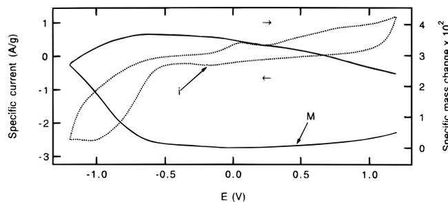
**Figure 6.** Specific current (current/sample mass) and specific mass (mass change/sample mass) as a function of applied potential for a nanotube film in 0.1 M LiClO<sub>4</sub> in acetonitrile, scan rate 50 mV/s (reference electrode Ag/Ag<sup>+</sup>).
