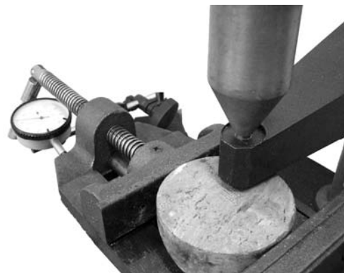
Figure 6 - Cerchar test apparatus
