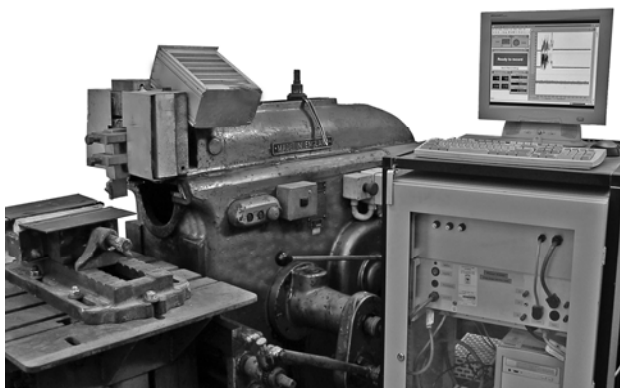
Figure 5 - Linear rock cutting machine
