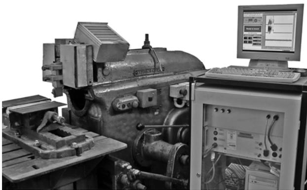
Figure 5 - Linear rock cutting machine
