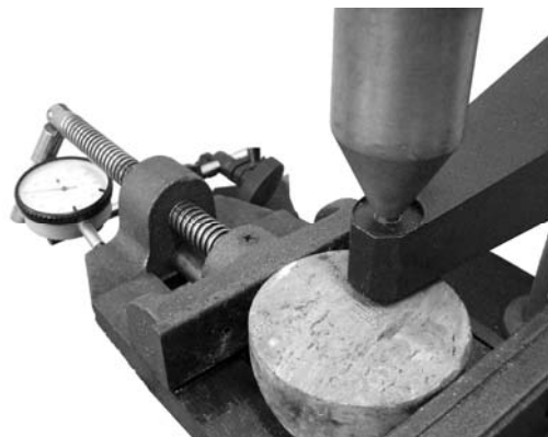
Figure 6 - Cerchar test apparatus
