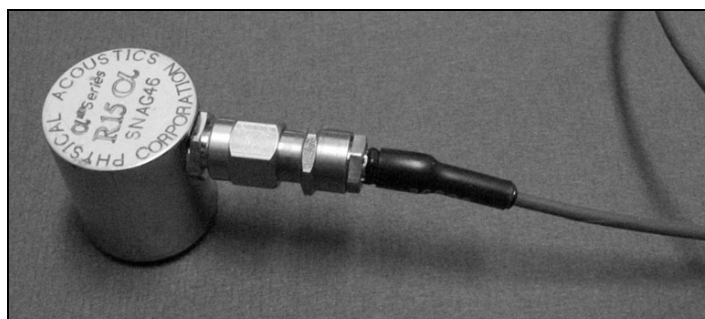
Figure 2 - The AE transducer sensor, model R15 \alpha
