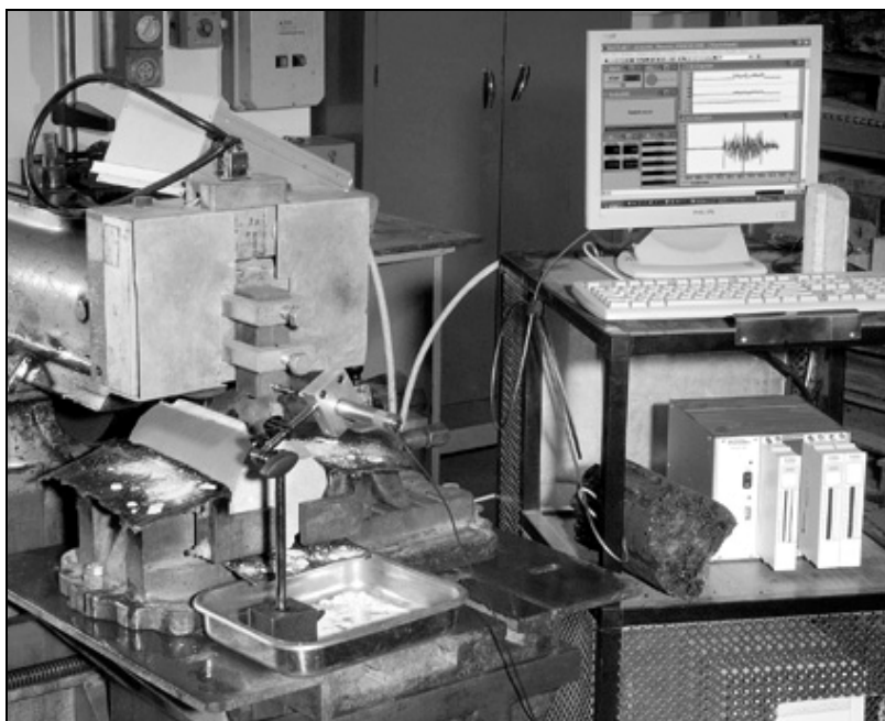
Figure 1 - Linear rock cutting machine used in cutting tests
