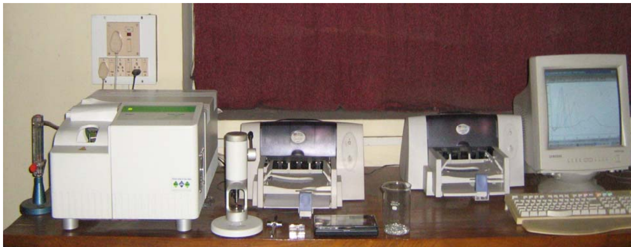
Figure 1 - Experimental setup of Differential Scanning Calorimetry
