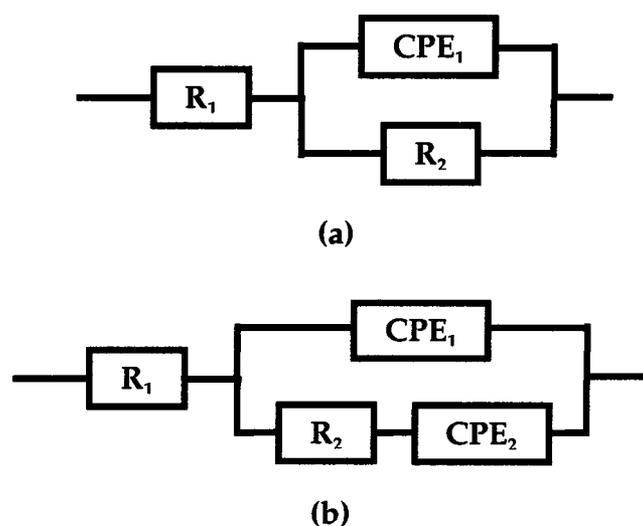
**Figure 2.** Equivalent circuits for (a) annealed and (b) unannealed CNT paper electrodes.  $R_1$ : resistance composed of solution resistance ( $R_s$ ) and electrode resistance ( $R_e$ ),  $R_2$ : charge-transfer resistance across electrode/solution interface,  $CPE_1$ : constant-phase element representing interfacial capacitance,  $CPE_2$ : constant-phase element representing pseudocapacitance from surface functional groups.
