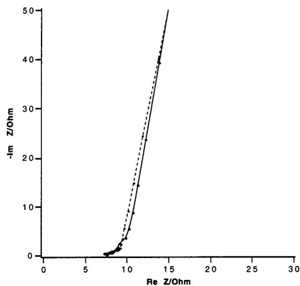
**Figure 3.** Nyquist plots for (a) annealed and (b) unannealed CNT paper electrodes at 0.0 V in 1 M NaCl showing experimental data (solid line) and simulated curves (dotted line) obtained from the equivalent circuits (Fig. 2).
