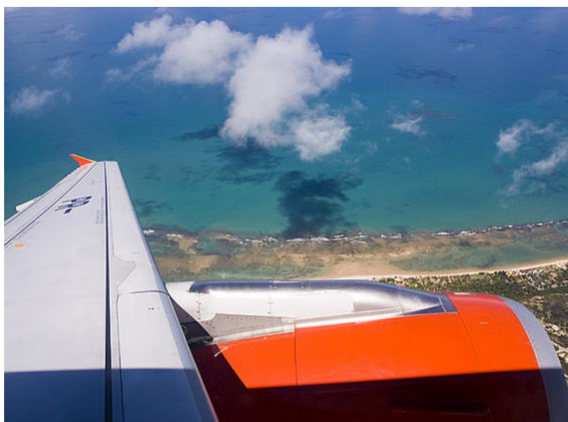
Figure 2 – Leading edge of an aeroplane wing showing no paint wear (Airliners.net website, 2008)
