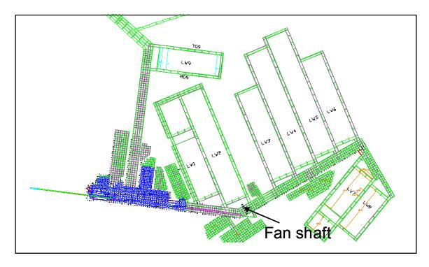
Figure 1 - Longwall layout plan for the first 9 Panels
