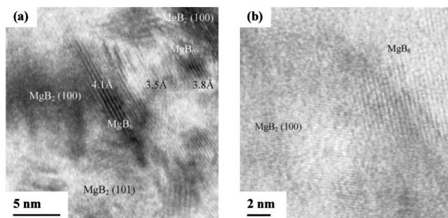
FIG. 2. (a) HRTEM micrograph exhibits smooth variations of lattice fringes with a range of 8.5 nm and a number of  $\text{MgB}_2$  lattice fringes are discernible. (b)  $\text{MgB}_2$  formed beside the nonequilibrium  $\text{MgB}_6$  observed in the other area.
