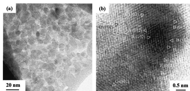
FIG. 1. (a) HRTEM micrograph showing that the MgB<sub>2</sub> grains consisted of a cluster of subgrains and the grain boundary of the adjacent MgB<sub>2</sub> grains was constructed by the boundaries of subgrains. (b) HRTEM micrograph reveals the nanostructural characteristics of the MgB<sub>2</sub>, which a nanodot was surrounded by nanodomains with small angle boundaries.
