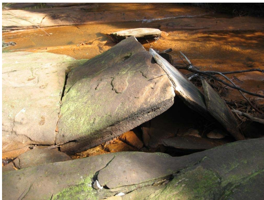
Figure 2 - Buckling of near-surface, Waratah Rivulet, late 2004
