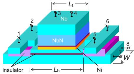
FIG. 1. (Color online) Schematic view of the multiterminal device. Electric current through the top (injector) junction can be fed through the contacts 1 or 2 (or 5 or 6) and 3 or 4. Bottom (acceptor) junction can be current-biased using the contacts 1 and 2 (or 5 and 6) and 7 and 8.
