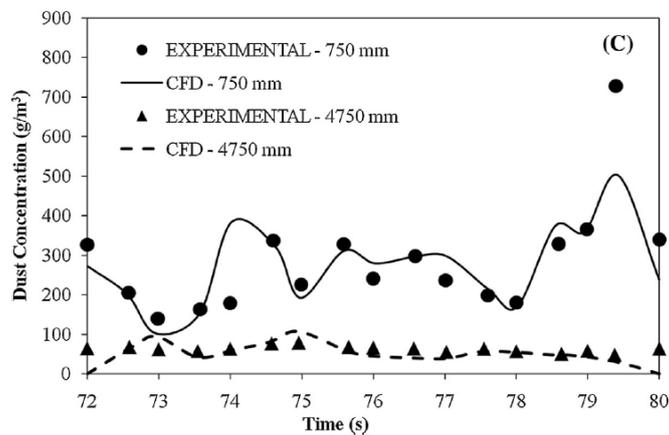
**Figure 5** Comparison Of Dust Concentration Data Points Between Rani *Et Al.* [56] And Hauert And Vogl (Adapted From [56])
