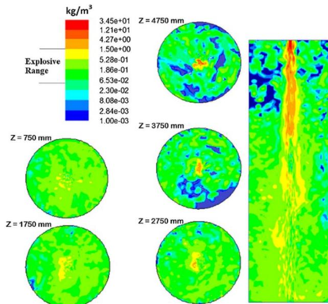
**Figure 6** Dust Concentration At Different Silo Heights Key Corresponds To Corn Starch Concentration (Adapted From [56])
