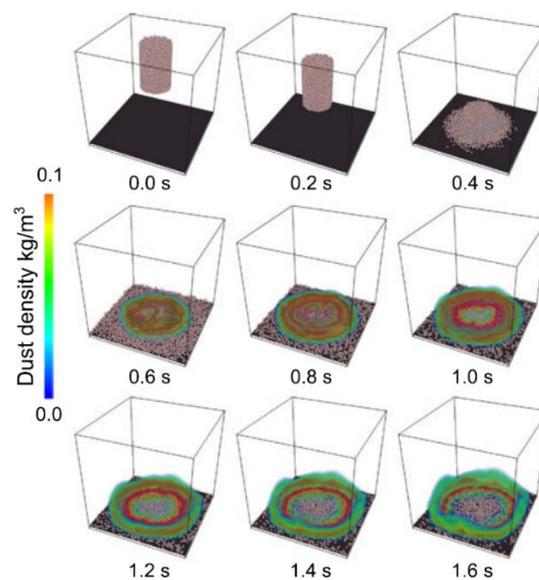
**Figure 4** Dust Generated By Falling Column Of Particle Of 2cm Diameter Dropped 0.5m Onto Flat Plate (Adapted From [54])
