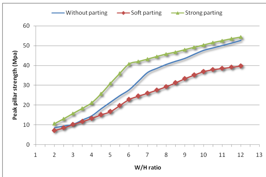
Figure 9 - The effect of the parting on coal pillar strength in FDM modelling
