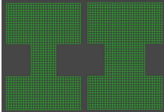
**Figure 1 - Modelled coal pillar with 3.0 m (10 ft) height and different widths**
