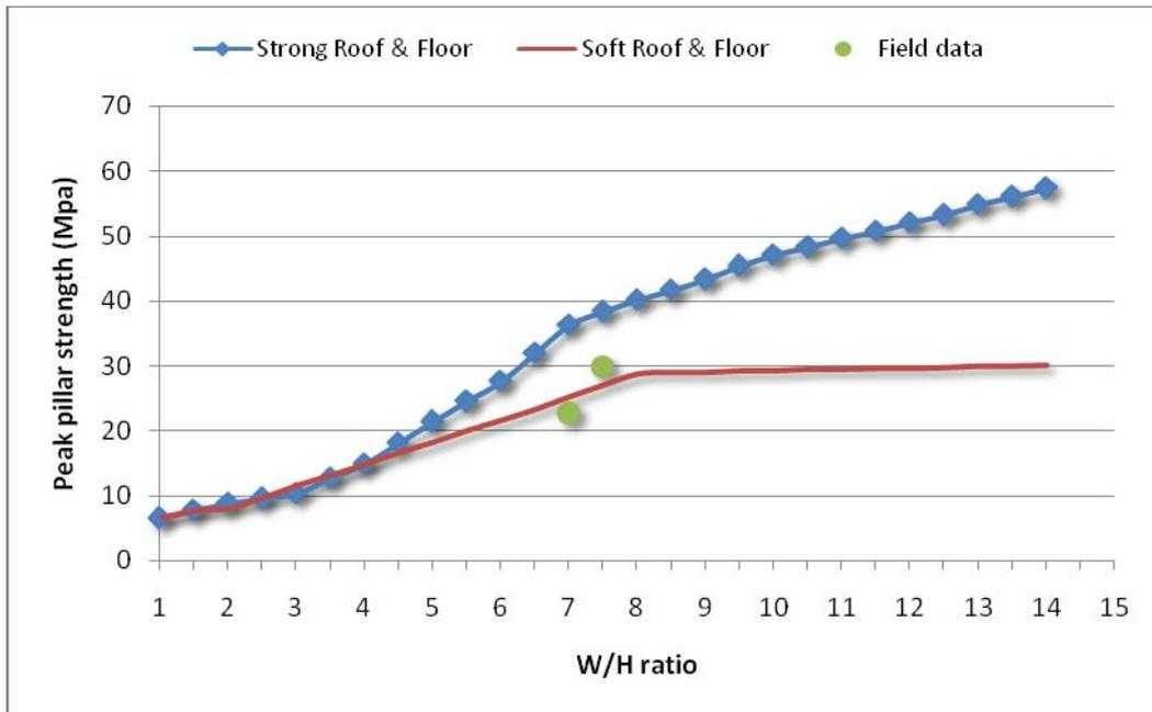
Figure 5 - The effect of surrounding roof and floor strength on coal pillar bearing capacity and comparison the results of FDM modelling with field data
