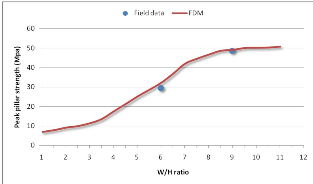
Figure 4 - The comparison results of FDM model and field data
