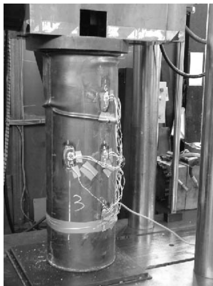
b) Continued buckling.
