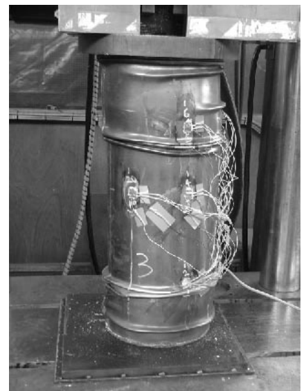
c) Continued buckling Can #3, 22% axial shortening.
