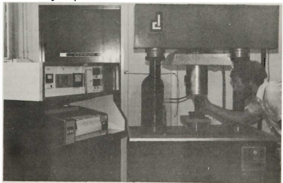
. The compression unit, capable of testing at elevated temperatures.
