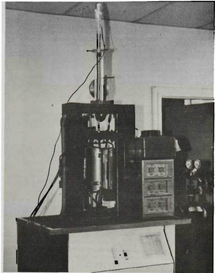
. The Tensile Unit, used to test materials in tension at high temperatures.
