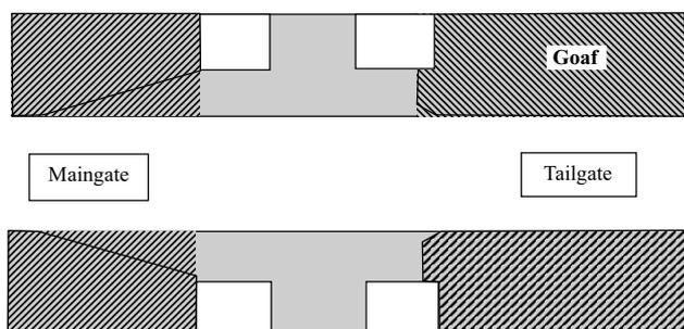
FIG 2 - Cartoon showing the location of gateroads in a thick seam relative to thicker seam extraction.
