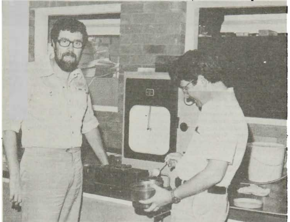
Professor S.A. Marshall (left) and Dr. P. Arnold in the Department of Mechanical Engineering's Flow Testing Laboratory. Dr. Arnold is putting samples into the Jenike Sheer Testing Machine.
