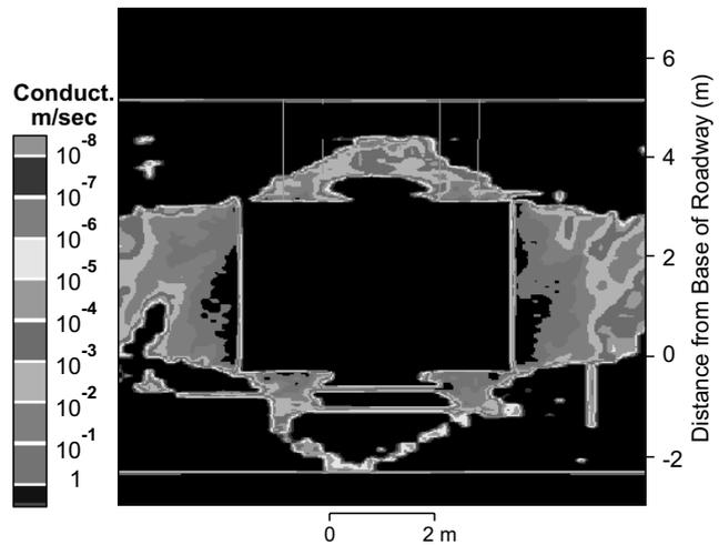
b) Conductivity about the roadway after 5 MPa abutment loading.
