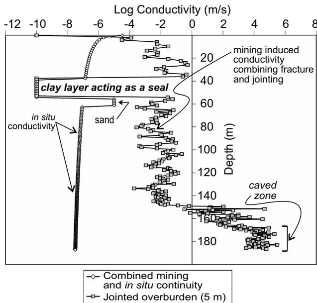
FIG 5 - Combined mining and *in situ* conductivity.
