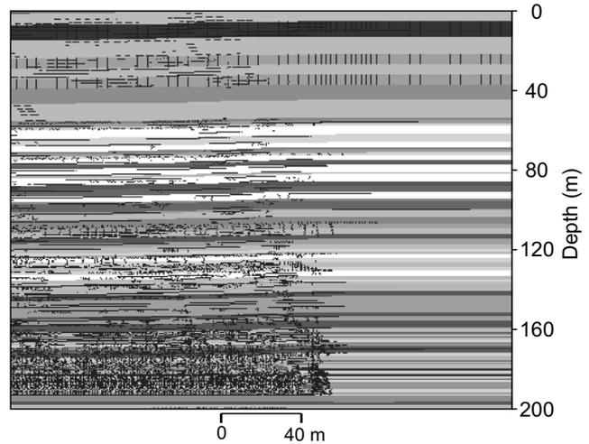
FIG 2 - Example of fracture distribution within strata layers.
