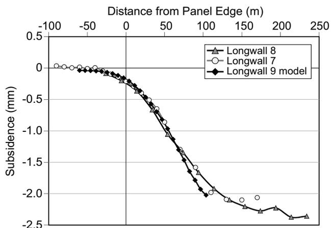
FIG 3 - Correlation of measured and modelled subsidence.
