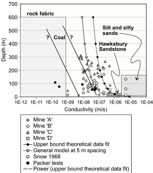
FIG 1 - Conductivity of individual rock fabric and jointed rock mass as measured from borehole testing.
