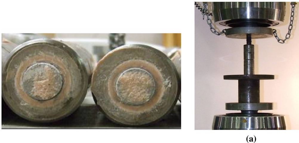
Fig. 1- (a) Uniform resin annulus thickness around the bolt (b) Push test arrangement, 150 mm sleeve
